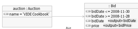
Figure 2. QQBE expression with a tuple result consisting of two named fields (“get dates and prices of bids placed for ‘VIDE cookbook’ between the given dates”).
